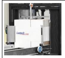
The blank magazine is provided with side curtains and transparent top guarding, mounted on the upper separator. The curtains will move with the adjustment on the blank magazine, in order to prevent entrance in the machine.
